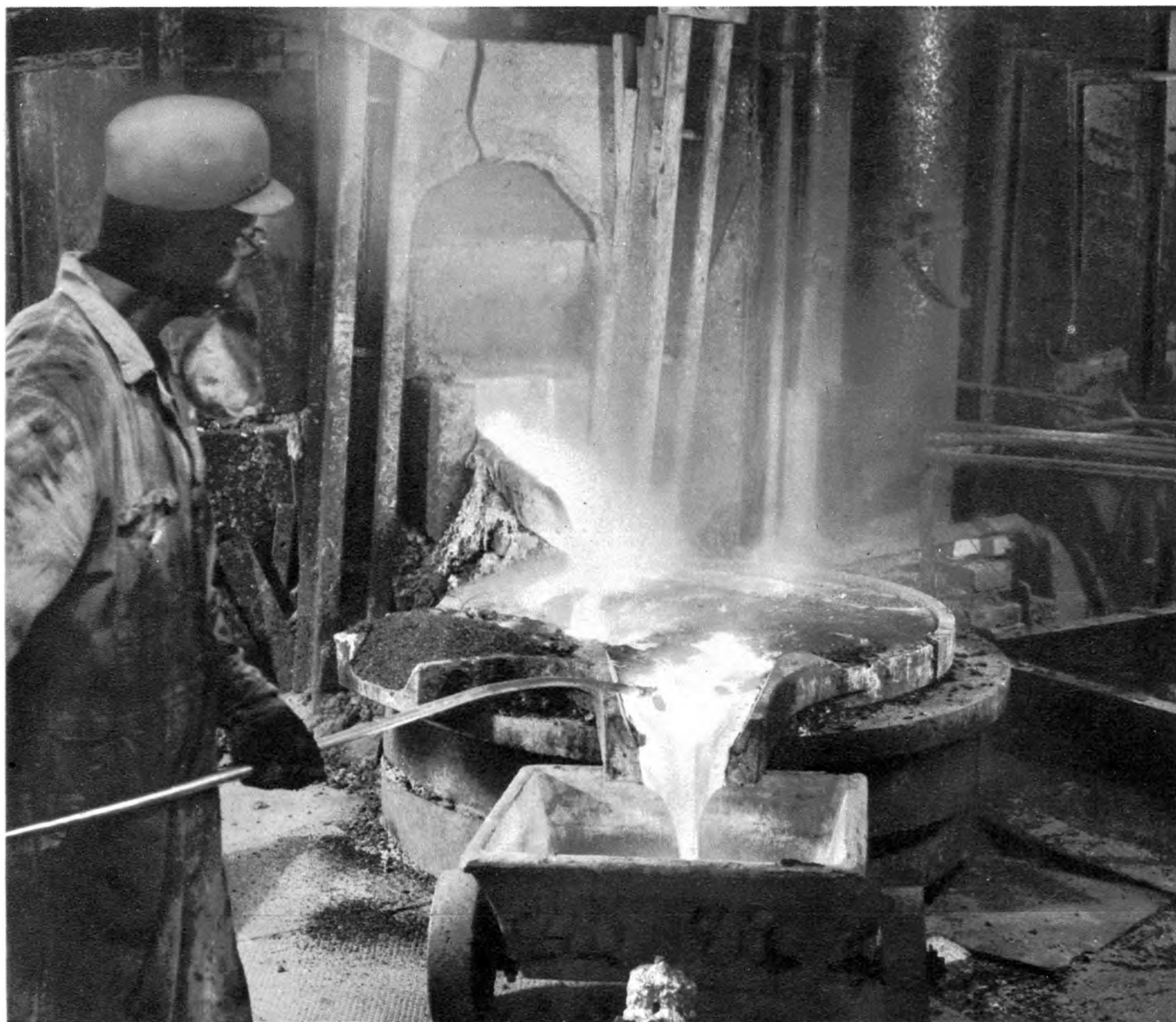
MELTING SCRAP LEAD from discarded telephone cable. It is smelted and refined at a Western Electric plant for reuse as cable sheathing.
